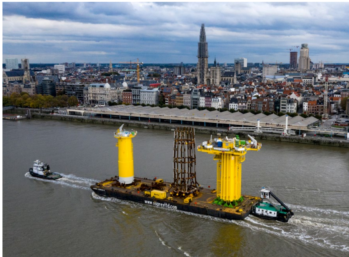
BELGIUM A touch of the SeaMade Offshore Wind Farm coloured the Antwerp skyline when the transition piece for the offshore substation was transported to Rotterdam for load-out
