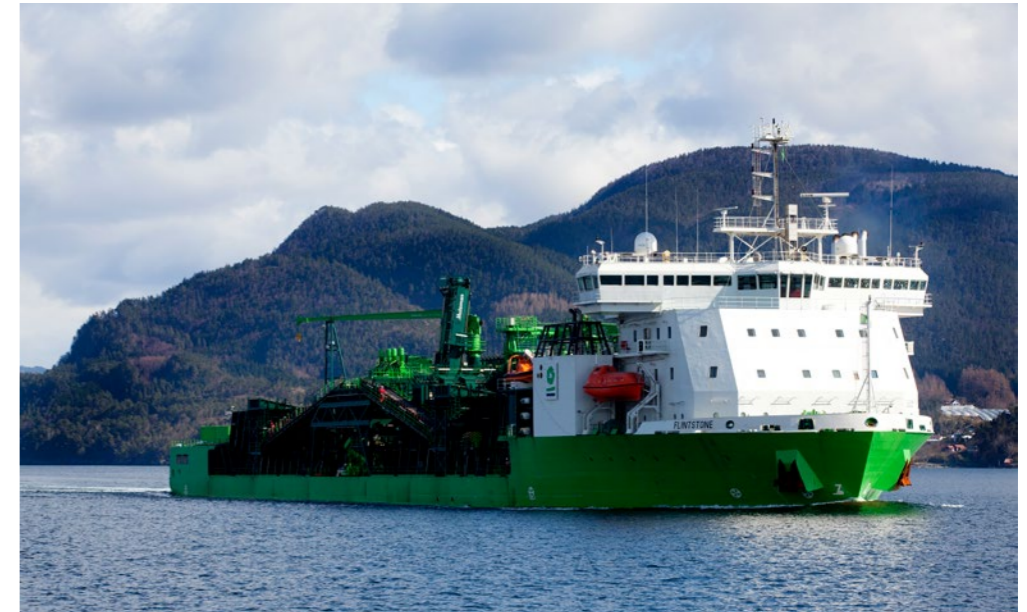
NORWAY DP2 fallpipe vessel 'Flintstone' worked several months in Norway for the NordLink and North Sea Link projects
